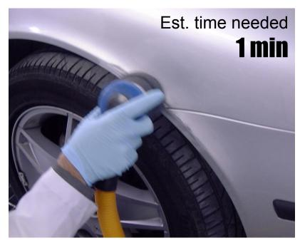
Use P150 - P280 to sand the surface to be repaired
