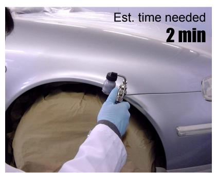
Apply the water based base coat
