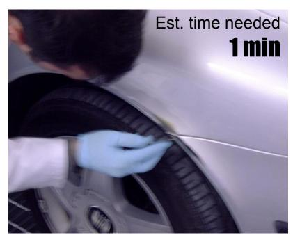
Fill the damaged area with the **UV-A1 Filler** (L19009)
