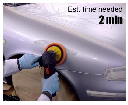
Polish the surface to totally eliminate the repair markings
