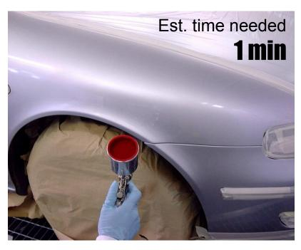
Apply the second coat of the **UV-A1 clear coat** (L19010) thinned at 10% with the **UV-A1 Thinner** (L19007) by Paintgun or Aerosol (L19010)
