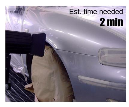
Wait 15 min and expose to the UV lamp for 2 min
