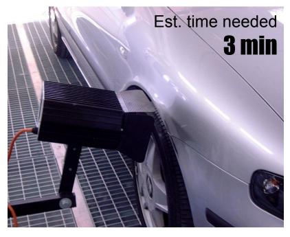
Expose to the UV lamp rays for 3-4 min depending on the thickness 10 cm distance (400W UV lamp)
