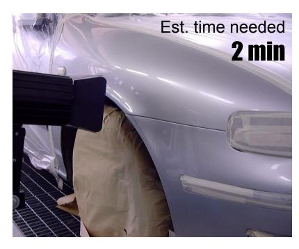
Wait 1 min (solvent base) or 2 min (water base), and expose to the UV lamp for 1 min.
