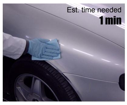
Degrease to eliminate impurities using Silicone remover
