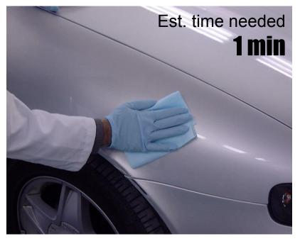
Degrease to eliminate impurities using Silicone remover
