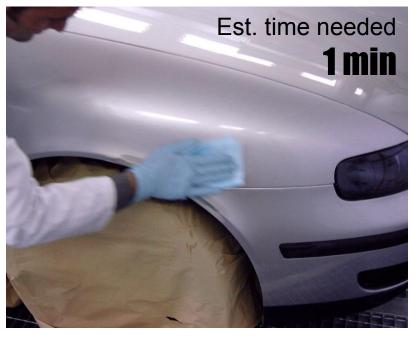
Degrease to eliminate impurities using Silicone remover
