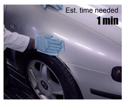
Degrease to eliminate impurities using Silicone remover
