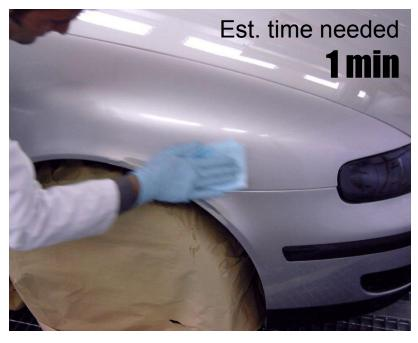
Degrease to eliminate impurities using Silicone remover
