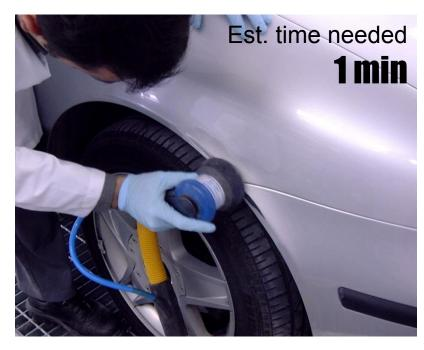
Sand the filled surface with P180 – P280 Refinish with P360 – P400
